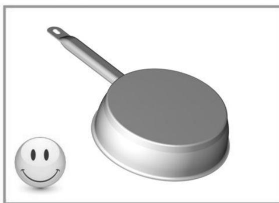
If the bottom of the pan ( $\varnothing d$ ) is significantly smaller than the diameter of the body ( $\varnothing D$ ) **the performance will not be good, and the pan might not be identified by the plate**
